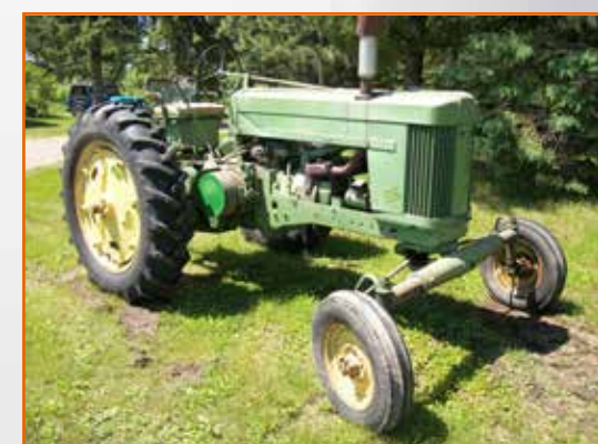
John Deere 60 wide front Gas eng, power steering, live 540 PTO, belt pulley, snl hydraulics, 13.6-38 rears -- one new, reads 7200 hours Ser # 6002219
