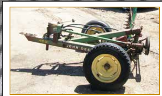
John Deere 450-9' sickle bar mower, PTO dr, Hyd lift, draw bar pull, on rubber
