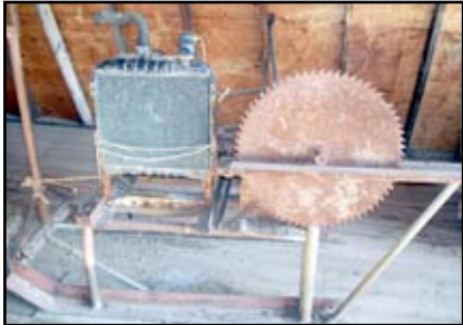
Home built saw rig 25" blade '53 Chrysler Simca "Flash" 4 cyl engine, ran good when last used.
