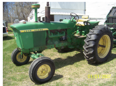
1962 John Deere 4010 diesel wide front ser # 20875 frnt and rear pto, 8.4X34 rears 80% 5665 hrs dual rear hyd, 3pt, PTO. Drawbar
