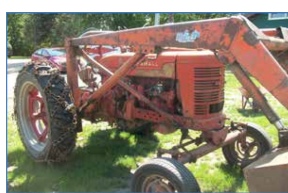
Farmall M wide front w/ Dual front end loader, PTO, pump, cast wheels 13.6-38 rears, good rear rubber & chains
