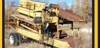
Tyler gravel screen w/3'x10' screens 20hp 3ph
