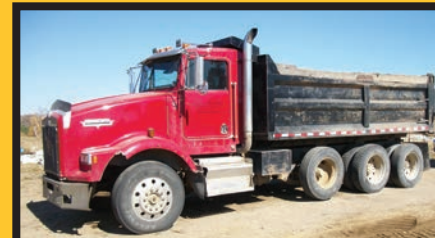
'90 Kenworth T800 dump truck w/14 yard box and tag axle, 425 CAT, 13 speed.
