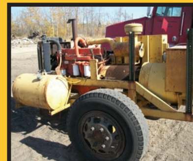
Generator 3 phase power unit w/4 cyl diesel, 230/460v 188/94 amp, approx 43K watt.
