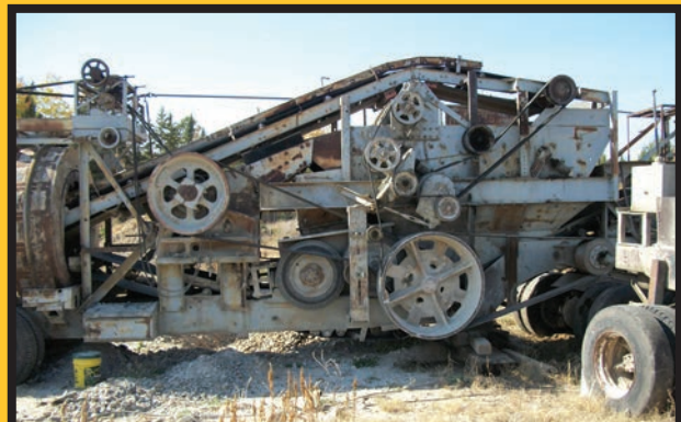
Cedar Rapids 1036 jaw and Roll Crusher, power unit for crusher 671 Detroit, Kolman feeder, Grizzly for crusher set at 10"
