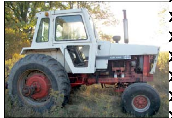
Case 1270 Agra King turbo tractor shows 5435 hours 4pairs hydraulic outputs, category 3 hitch 3pt 540 PTO 18.4x38 rears set up for duals but running singles for now.
