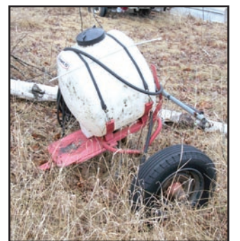
ATV pull type sprayer approx 50 gal
